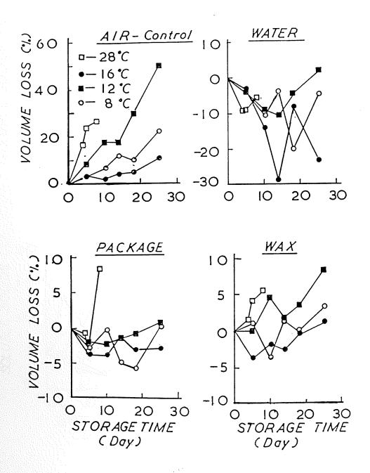
Figure 2: Volume losses of breadfruits in storage
