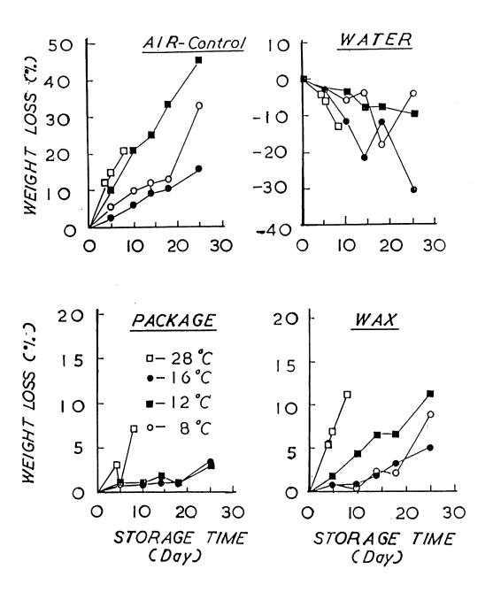
Figure 1: Weight losses of breadfruits in storage
