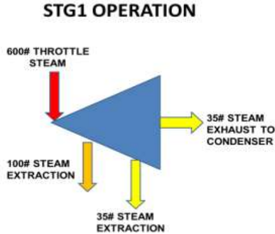
Figure 6: STG1 Steam Schematic
