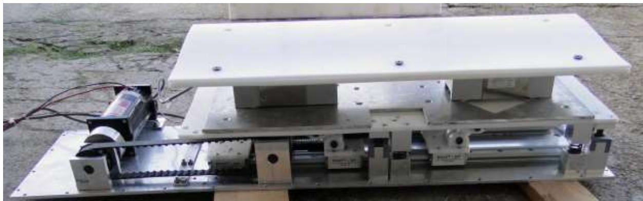
Figure 2: Prototype of the road pavement energy harvesting system.
