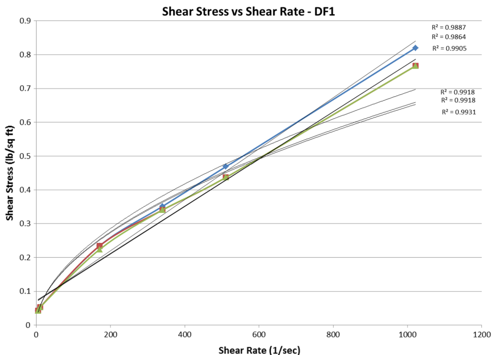
Fig. 4 Rheological plot for DF1 showing best fit curves and correlation coefficients
