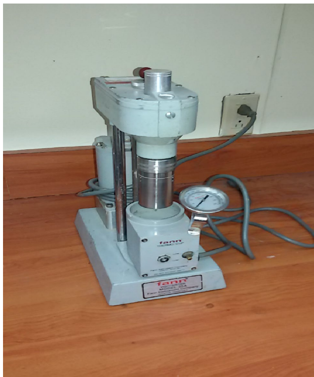
Fig. 3 Typical Fann Model 35 Viscometer
