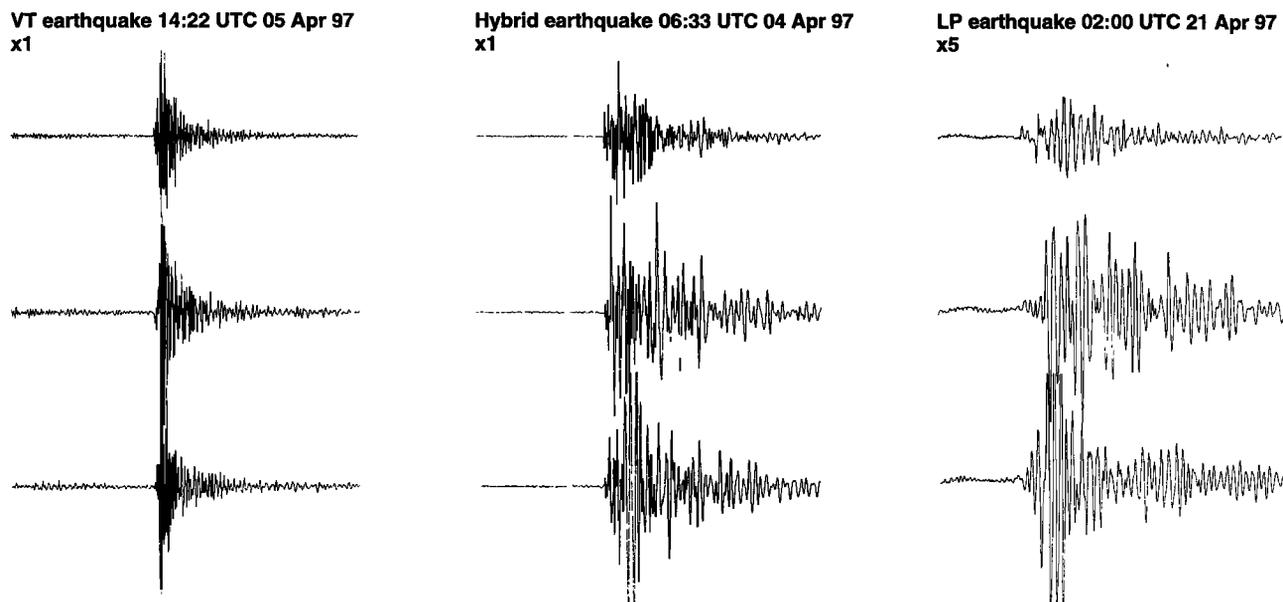
Figure 1. Examples of seismic signals from the Soufriere Hills volcano. Vertical, north-south, east-west components recorded by the Gages broadband seismometer (see Aspinall *et al.*, 1998 for location).
