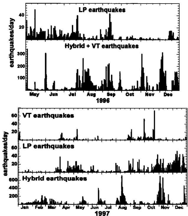
**Figure 3.** Daily counts of VT, LP, hybrid earthquakes between May 1996 and December 1997. The 1996 data are for earthquakes which triggered the analogue network recording system (Aspinall *et al.*, 1998), when VT and hybrid earthquakes were not discriminated during classification. The 1997 data come from the digital network (Neuberg *et al.*, 1998).
