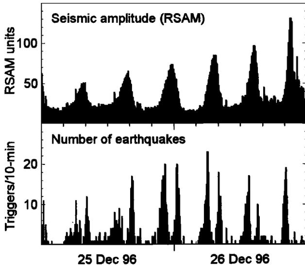
**Figure 2.** Signal amplitude (top) and number of earthquakes (bottom) for the short-period seismometer at St George's Hill, 25-26 December 1996. Episodes of small, repetitive hybrid earthquakes and tremor occurred every 8 hours. As the series progress, the episodes became close together and increased in intensity. Earthquakes occurred at the beginning and end of each episode, and coalesced to a continuous tremor signal in the middle.
