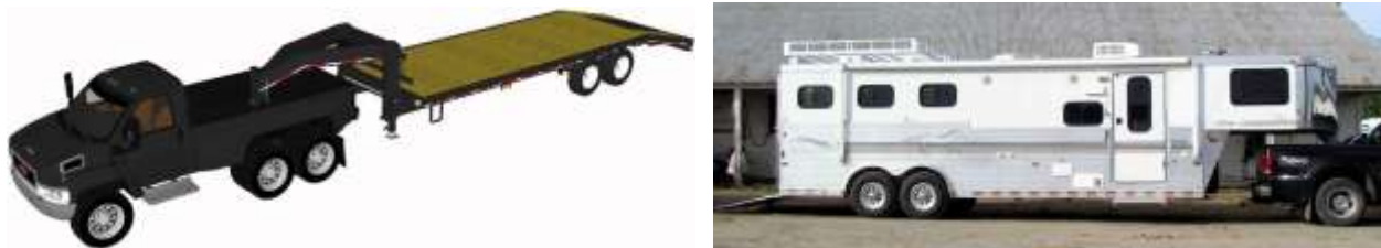
Figure 1: Examples of conventional gooseneck trailers attached to a pickup truck [en.wikipedia.org].
