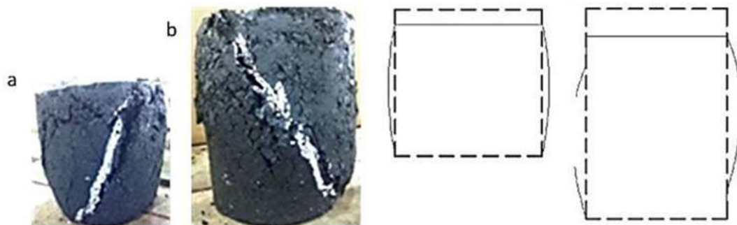
Figure 8: Failed test samples (a) 100 mm height (b) 150 mm height
