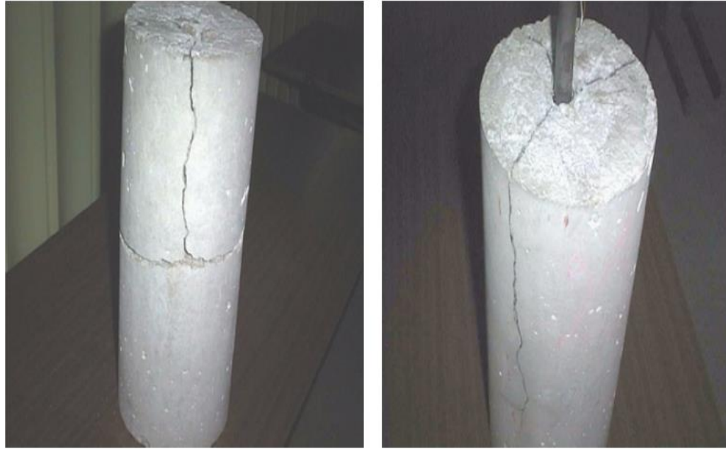
Figure 8: Concrete cylinder failing by splitting
