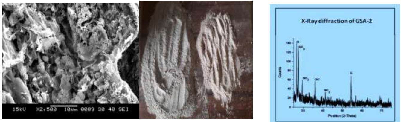
Figure 1.0: SEM images (at 2500 \times ), physical appearance of GSA resembling Portland cement and its XRD
