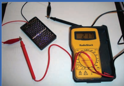
Prototype of the Solar Panel Tester developed by student Darrell Gordon, under the supervision of faculty Dr Paul Aiken.
