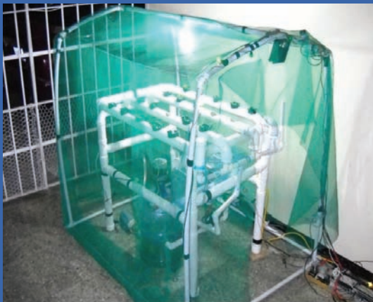
A model of the Renewable Energy Driven Microcontroller Based Fully Automated and Controlled Hydroponic Greenhouse System in use.
