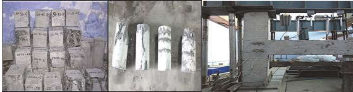
Figure 4: Beam-column joint specimen during testing
