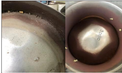
Fig. 8. The rusted underside of a Tenor and Three Cello.
