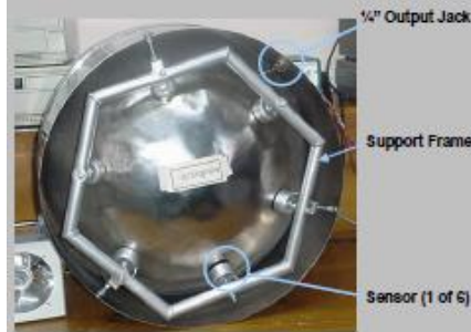
Fig. 30. Lectrapan magnetic frame and structure on a tenor pan
