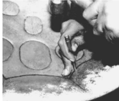
Fig. 9. Creating a groove on an outer note's inner boarder
