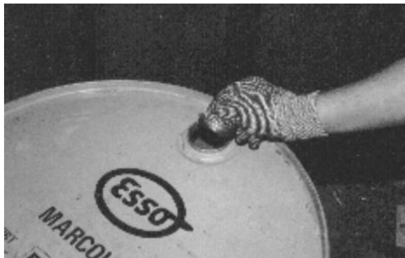
Fig. 2. The removal of the plug to allow air out during the sinking.
