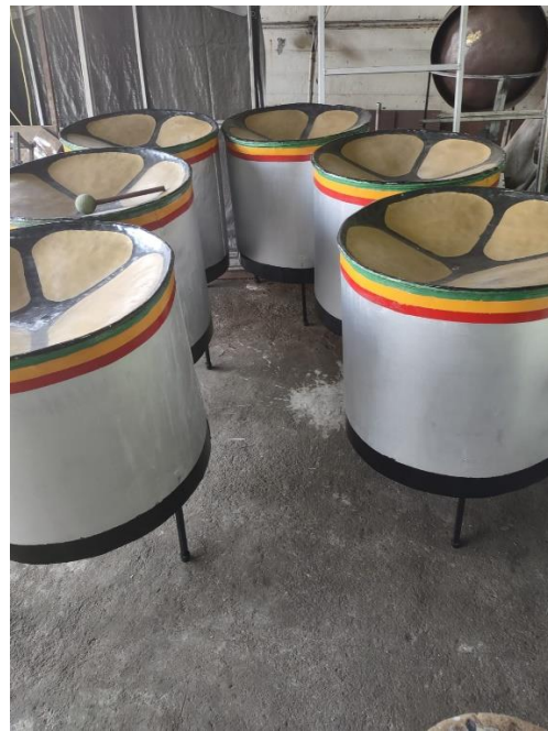
Fig. 14&15. Bases made from metal sheets.
