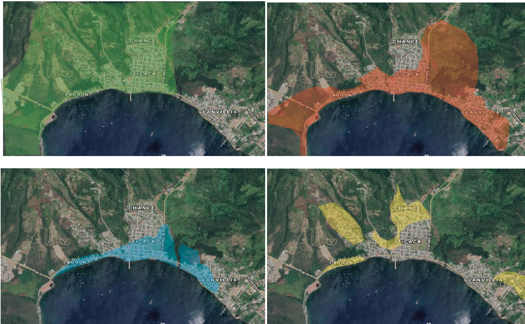
Figure 4. 19 Hazard risk map for Portsmouth showing selected hazards. Notes - green – volcanic; red – tsunami; blue – flood; yellow landslide.
