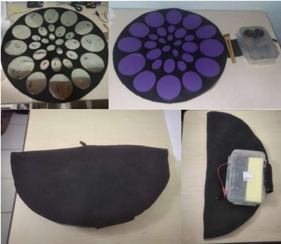
Figure 6: Design prototype of the roll-up digital steelpan constructed for testing
