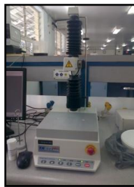
Picture 2 showing the Texture Analyser, TA.XT plus used for texture analysis of the patty.
