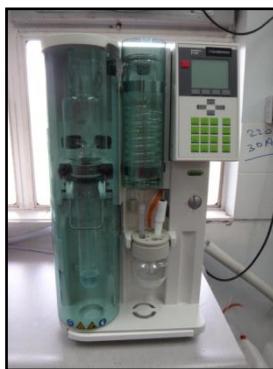
Picture showing the Kjelflex automated machine used for the extraction of crude protein from sample.
