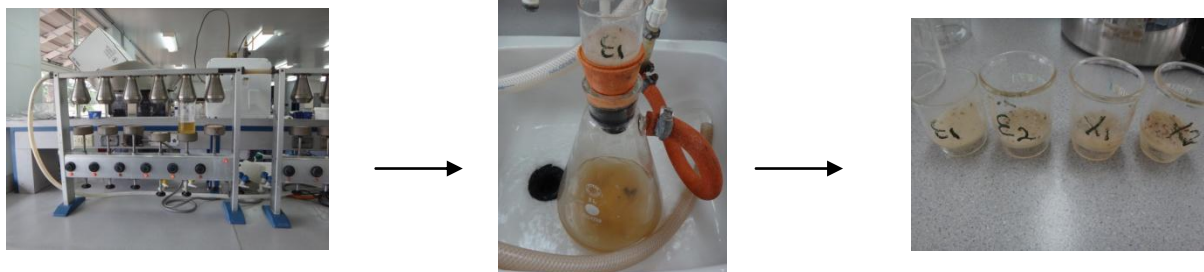
Pictures showing the equipment used to extract fiber and the gooch crucible used to filter and collect sample.
